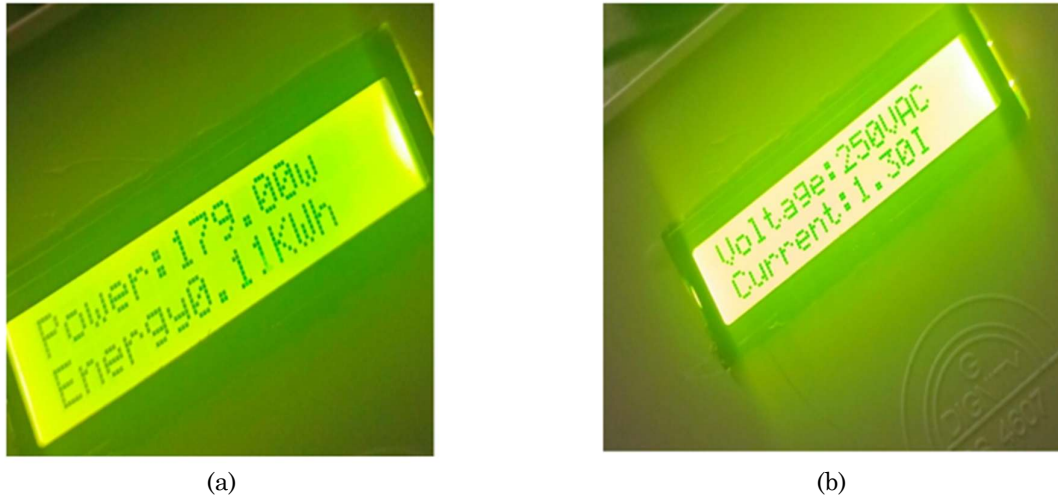
Fig. 5. Onscreen Display: (a) Power and Energy, (b) Voltage and Current
