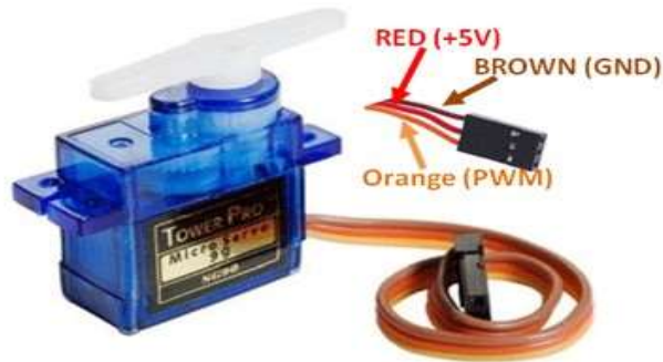
Fig. 10. Micro Servo Motor SG90 Pinout Diagram
